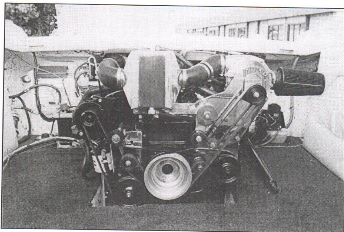
FIGURE H1 COMPLETED ProCHARGER SYSTEM INSTALLATION
