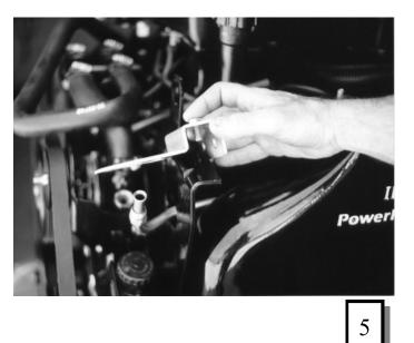
Feed oil line shown in fig. 4 through hole in original bracket.
