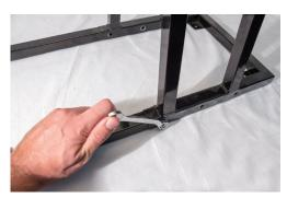
4) Install bolts with the button head on inside.
