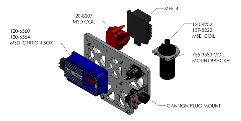
THESE ARE THE PARTS THAT CAN MOUNT TO THE BRACKET
