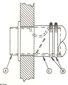
A-EXHAUST TIP B-HDSE CLAMP C-EXHAUST HDSE
