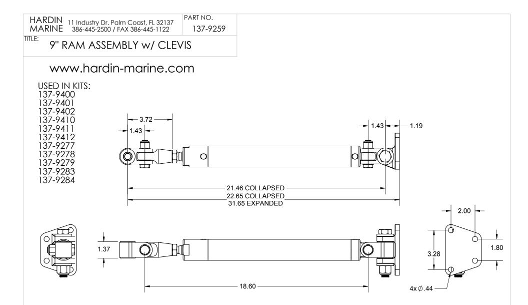
KIT COMES w/ 316SS 16 "HOSES, FITTINGS, THRU HULLS & MOUNTING HARDWARE, NOT SHOWN.
