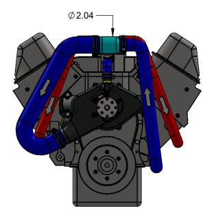
THIS IS A STANDARD RAW WATER THERMOSTAT HOUSING. THIS HOUSING ALLOWS WATER TO BE BYPASSED TO THE EXHAUST MANIFOLDS UNTIL THE THERMOSTAT OPENS. ONCE THE THERMOSTAT OPENS, ALL IN COMING WATER IS CIRCULATED THROUGH THE ENGINE BEFORE GOING OUT THE EXHAUST.
