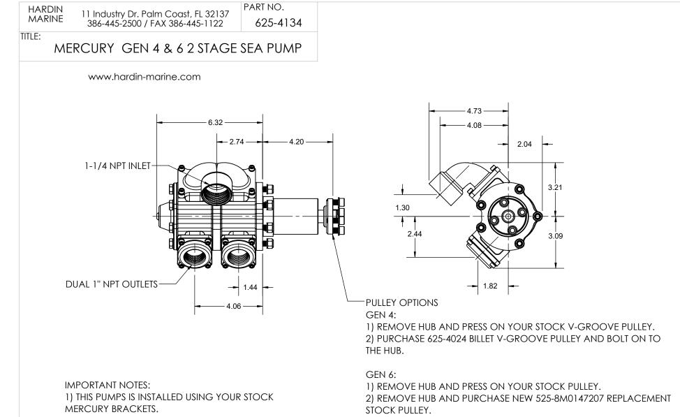
2) YOU CAN USE THIS PUMP TO REPLACE GEN 5, 525, 600 & 700 SEA PUMPS IF YOU ARE NOT USING THE FUEL PUMP.
