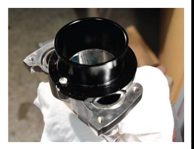
2. Grease the cone to allow the impeller to slide easily when rotated into the cone.
