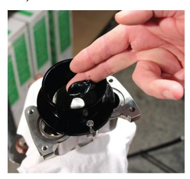
3. Place the impeller in the cone and then slide the impeller drive tool into the impeller.
