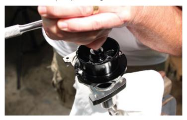
7. Now remove the installation cone and finish the rebuild on the pump.
