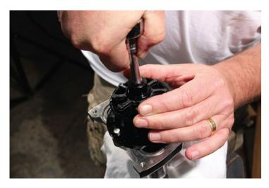
6. With the impeller flat aligned with the pump shaft flat press downward until the impeller is seated in the pump housing.
