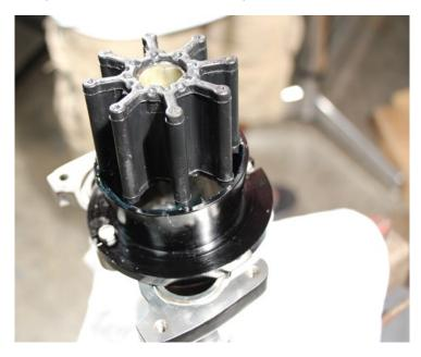
4. Using a 3/8" ratchet with a short extension placed in the square drive hole rotate the impeller anti-clockwise while pushing the impeller into the cone.
