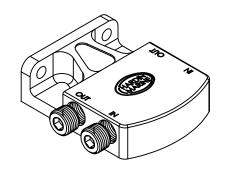
INLET/OUTLET PORTS ARE 1/2 NPT. SUPPLIED ARE 2 PIPE PLUGS. USE THREAD SEALANT ON ALL NPT THREADED HOLES.
