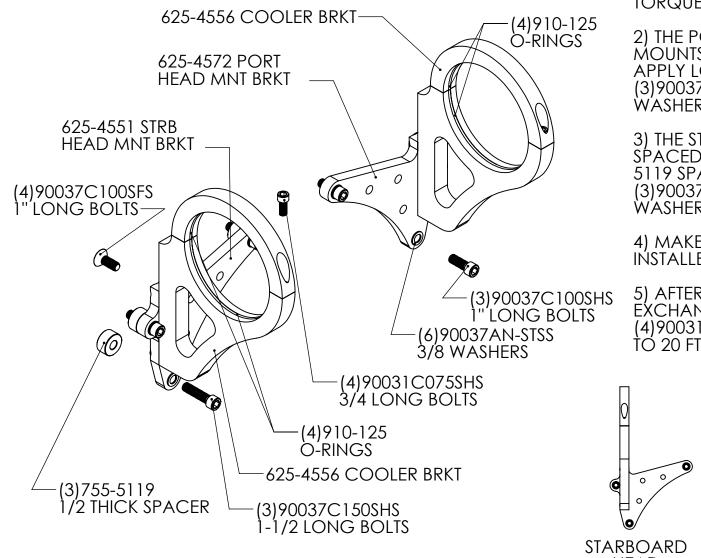
MOUNTING INSTRUCTIONS: 1)ATTACH 625-4556 OIL COOLER BRACKETS TO HEAD MOUNT BRACKETS. APPLY LOCTITE TO THE(4) 90037C100SFS **BOLTS & INSERT THROUGH THE** COUNTERSUNK SIDE OF THE BRACKET. TORQUE TO 30 FT. LBS...
