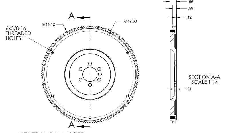
**NEUTRAL BALANCED BLOCK MOUNTED STARTER** ACCEPTS MERCURY COUPLERS AND HEAVY DUTY DRIVE PLATE. WEIGHT: 28 LBS... 168 TOOTH RING GEAR
